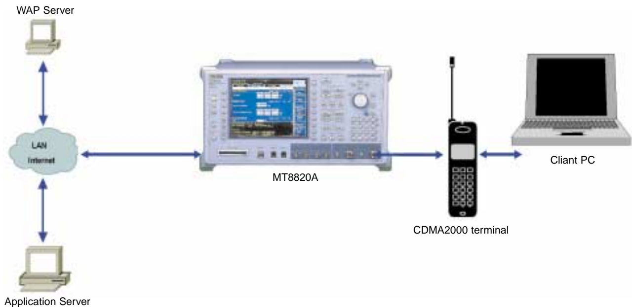
Example of IP Data Communications Mode
